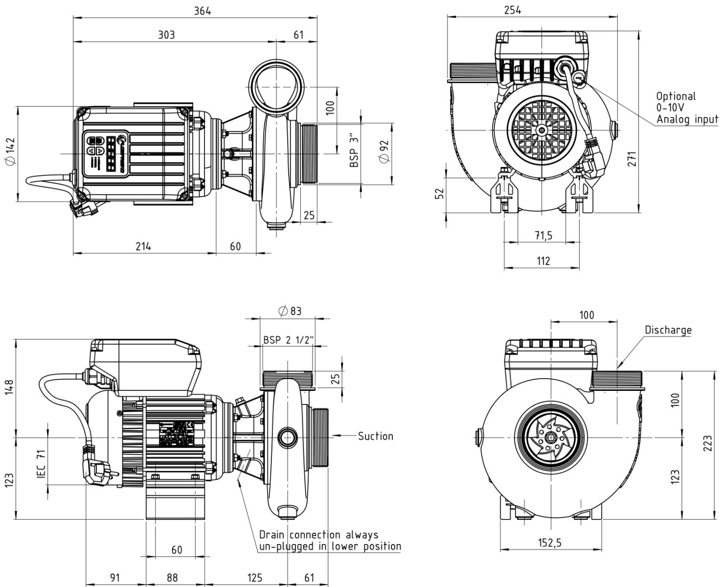
Pumpcasing can be rotated in steps of 45 degree.
